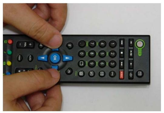
When under MCE mode, you can find the POWER key blinks every time you press on the remote control. However, in Standard mode, POWER key does not blink. You can also tell which mode the remote control is in by this way. The picture below illustrates the POWER key lights up when key on the remote control is pressed. (Please notice the lighted POWER key circled by the green MCE mark.
