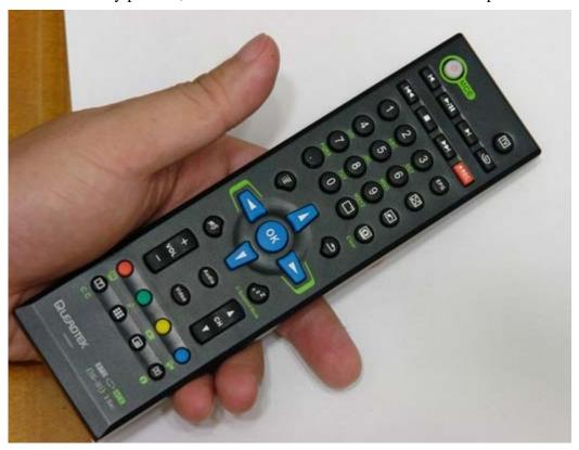
When under Standard mode, POWER keys does not blink no matter what. You can use this feature to tell which mode the remote control is in, and to make sure if the switch success or not.
